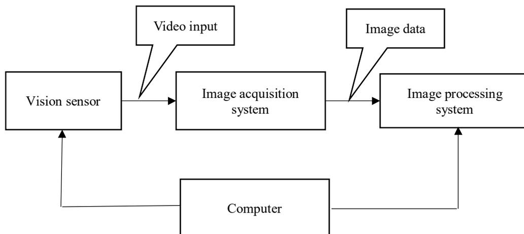
**Figure 1.** Machine vision system composition
