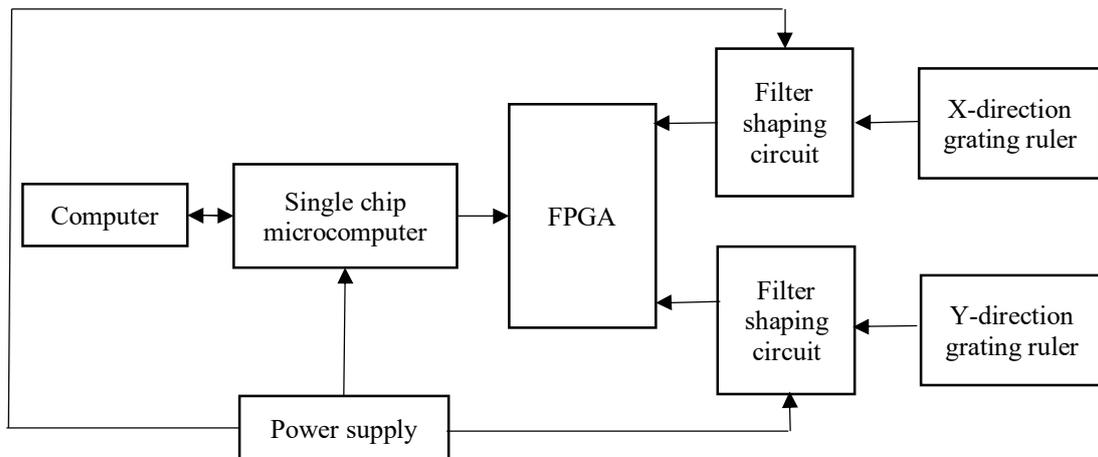
Figure 3. Raster signal processing module structure
