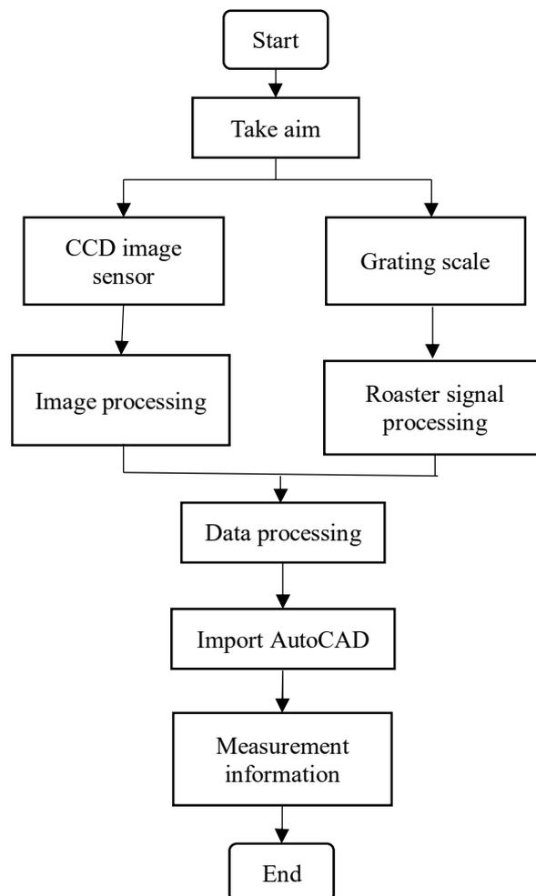
Figure 4. Measurement process
